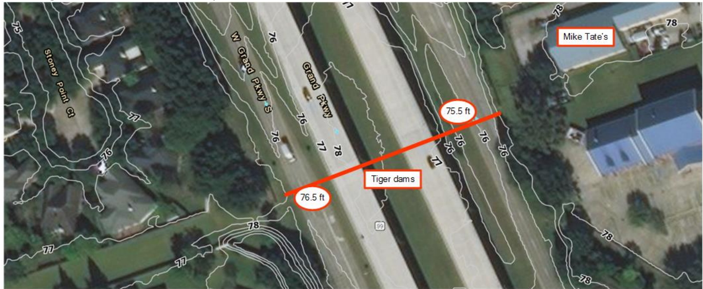
Max rain water height reached 76.5 ft at tiger dams.
